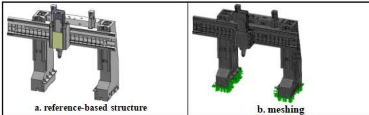
Fig. 2. Reference-based structure and its meshing
